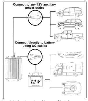
Amorphous solar panels convert daylight directly into 12V electricity. Suitable for maintaining charge in a wide range of batteries and power packs. Ideal for batteries stored in boats and caravans and for batteries in vehicles in long-term storage. IP44 Rating (non-waterproof). For use behind car windscreen or other protection. Supplied with battery clips and vehicle accessory socket plug (only suitable for vehicles with "permanent live" accessory socket).
